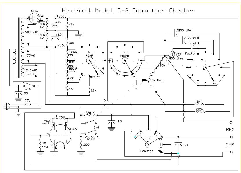
S-1 is rear section main switch. S-2 is front section of main switch. S-3 is Leakage switch. S-4 is on rear of Power Factor Control. S-5 is power switch, mounted on rear of main switch. All switches, except S-4 shown in normal ( $\Box$ ff) posistion.
